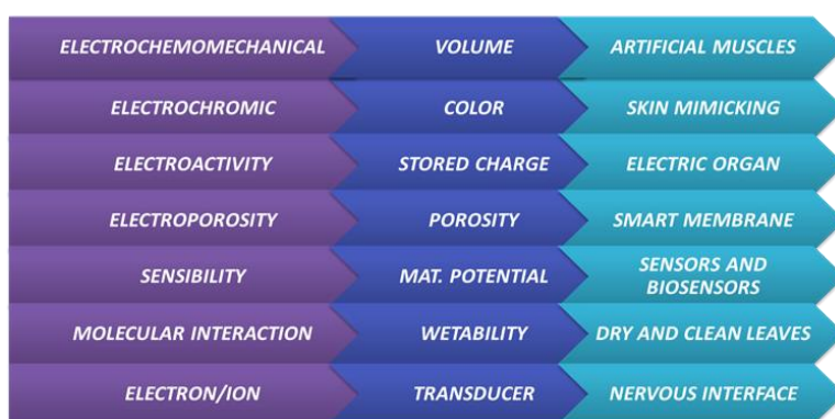
Figure 1.9 Biomimetic properties of CPs driven by the electrochemical reaction, the mimicked biological functions and the related organs
