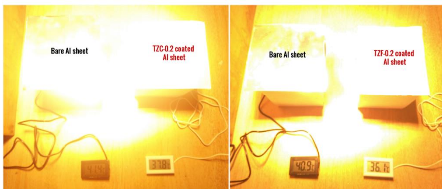
Figure 6.22 – Difference in interior temperatures observed after thermal shielding studies using a) TZC-0.2 and b) TZF-0.2 coated Al sheet roofing in comparison with bare Al sheet roofing.
