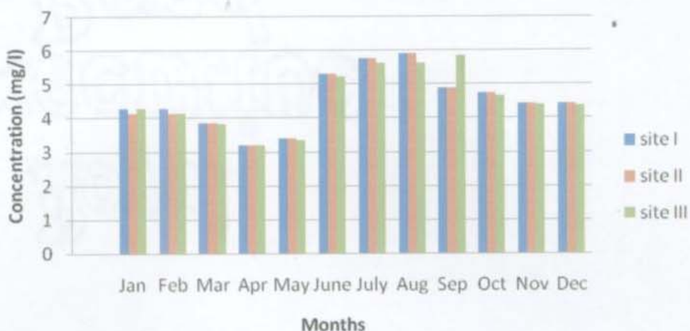
Fig. 16. Seasonal variation in the dissolved oxygen content of the three sites during 2005-06
