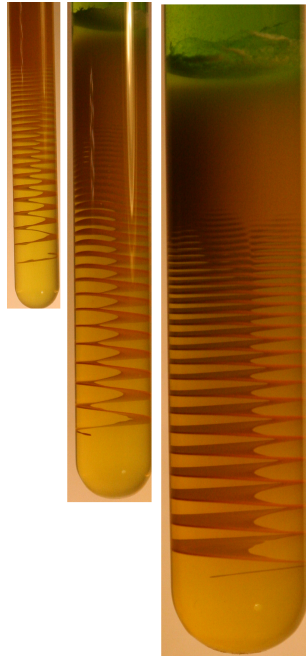
Figure 3.6: Helical patterns in agarose gel having test tube diameters 8mm, 12mm, 18mm
