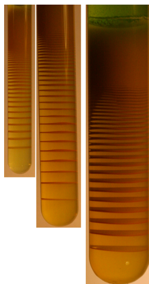
Figure 3.5: Liesegang patterns in agarose gel having test tube diameters 8mm, 12mm, 18mm
