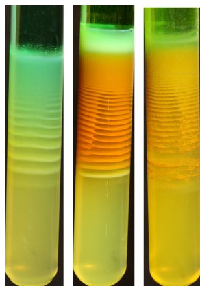
Figure 3.13: Effect of impurity on patterns- 10 ml agarose, 50 ml agarose, 80 ml agarose in silica are shown
