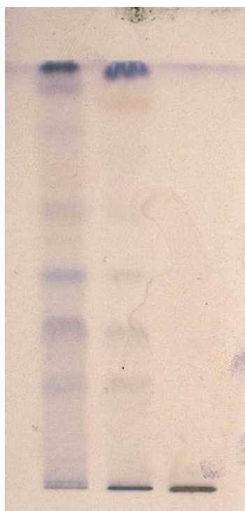
Fig 35 :HPTLC image after derivitization observed at 550nm
