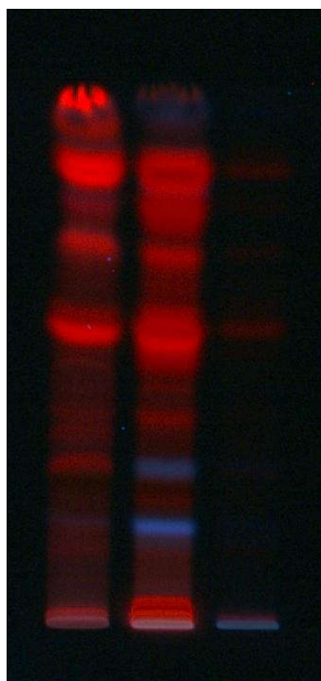
Fig 75: HPTLC image after derivitization viewed at 366nm
