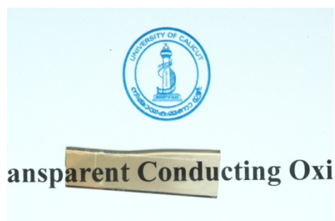
Figure 4.24 Actual photograph of \text{SnO}_2 film sputtered at 150^\circ\text{C} and 120W
