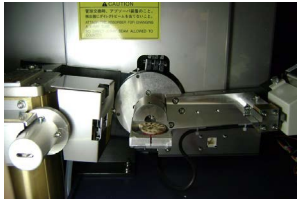
Figure 3.1(a) Schematic illustration of diffraction process and (b) Internal view of the X-ray diffractometer
