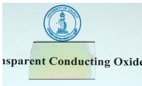
Figure 4.41 Actual photograph of ITO films sputtered at 120W and 100°C
