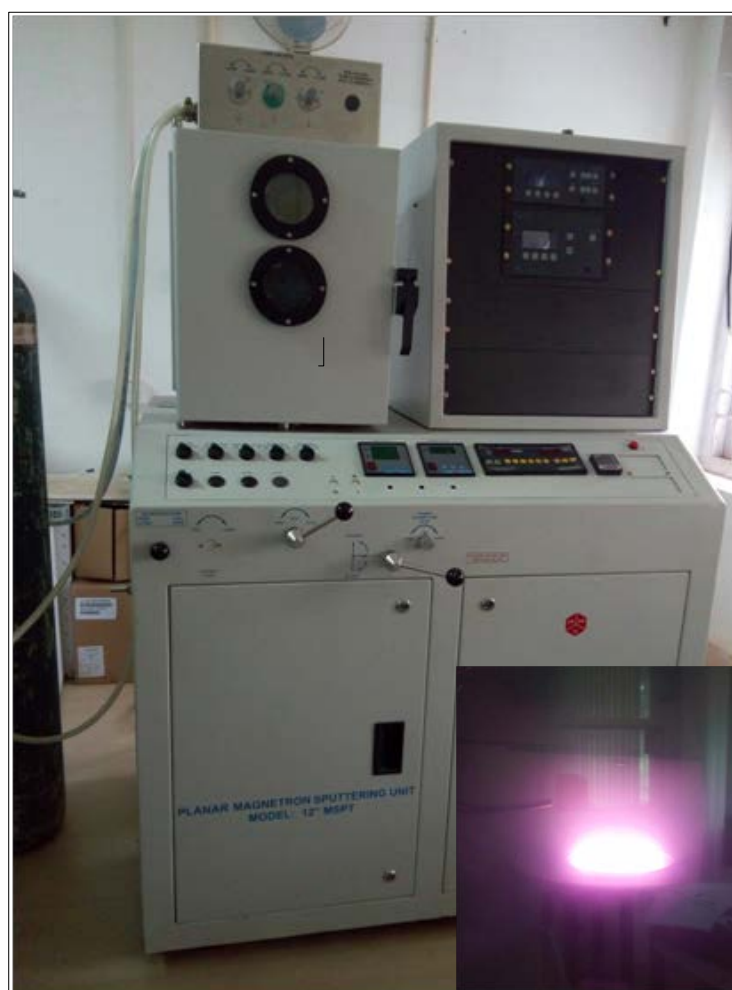
Figure 2.2 Radio frequency magnetron sputtering set up. In the inset, plasma formed during the coating of ITO films.
