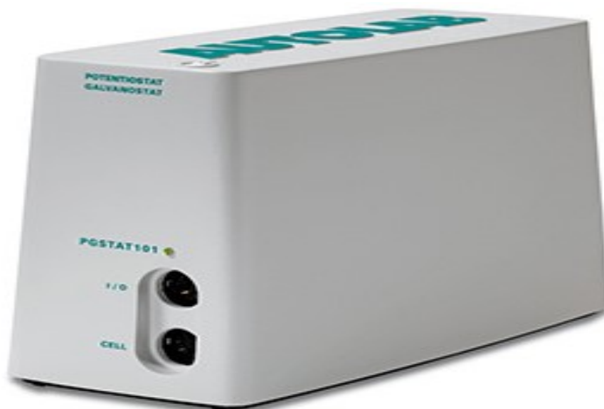
Fig. 38 AUTOLAB 50519 PGSTAT instrument used for impedance measurements
