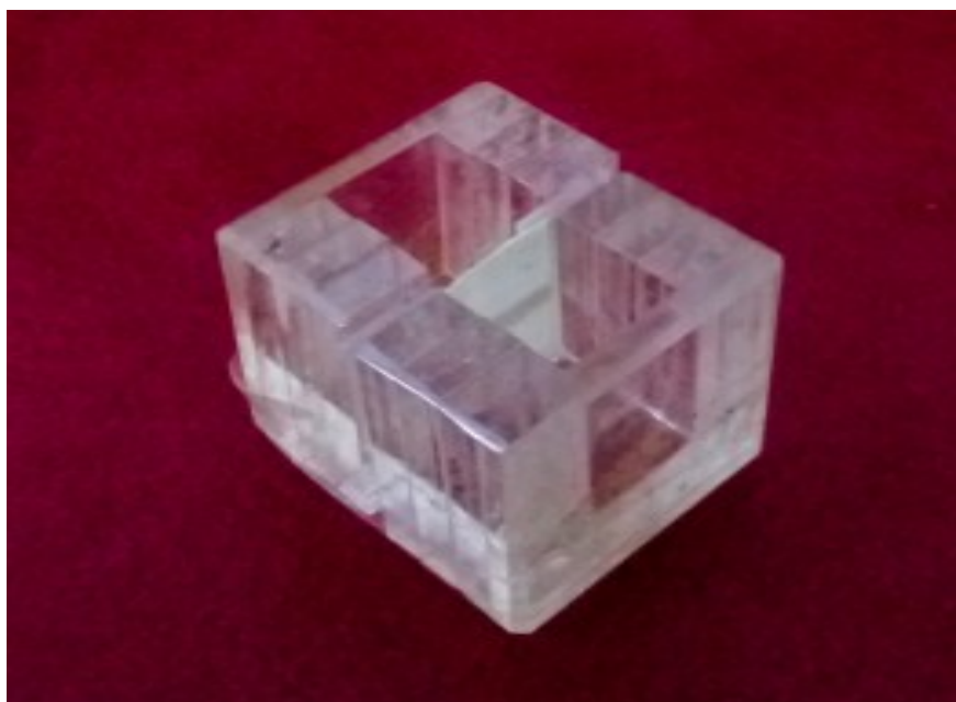
Fig. 39 Conductivity cell used for the impedance measurements
