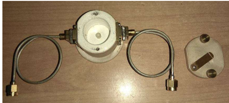
Figure 2.12 Cavity setup for the measurement of Q-factor
