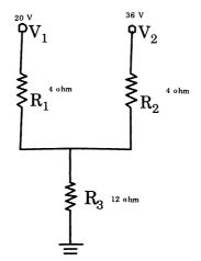
31. Using Kirchoff's law calculate the branch currents in the network of figure given below.
