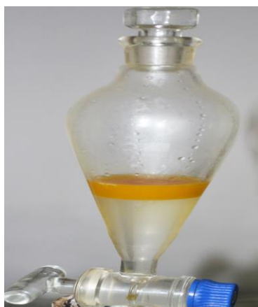
Figure 3.8. Purification of biodiesel with hot water treatment.
