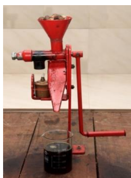
Figure 3.2. Mini handed oil expeller
