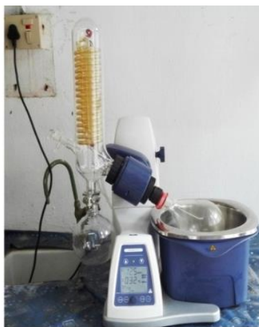
Figure 3.4. Separation of oil using rotary evaporator.
