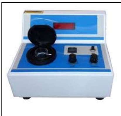
Figure 5.9: Image of Turbidimeter used for quantification of \text{Pb}^{2+} ions(LABTRONICS LT-33 Digital Turbidity Meter)
