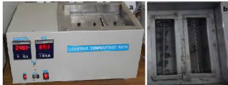
Figure 3.2: Chemical etching set up
