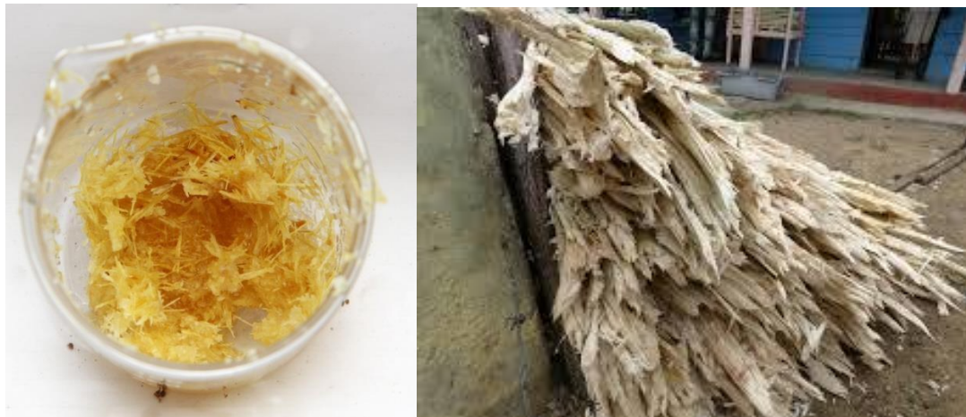
Fig.14 Bagasse raw and delignified- enormous quantities of this material is burnt in the field. This material being lignocellulosic can be used for the production of microbial metabolites , including Bti
