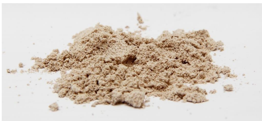
Fig.18. Taro powder- milling or powdering increases surface area which in turn increases the assimilability of the raw material by the microbial enzymes.
