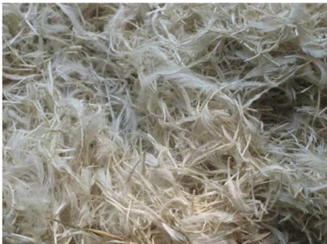
Figure 25: Poultry feathers after Methanol: Chloroform treatment
