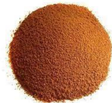
Fig.22 Ferric chloride ( commercial grade) which is cheap and readily available used as a flocculant . Flocculation of Bti cells will substantially reduce filtration/centrifugation time and costs both of which are power intensive operations in the down stream operations in biotech industry. Effect of Aluminium sulphate on filtration of the fermented broth of Bacillus thuringiensis var israelensis
