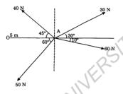
(a) Determine the resultant of the force system as shown in figure with respect to point O. All squares are unit squres.
